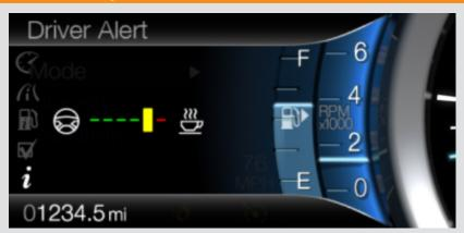
The Driver Alert System is designed to help alert drowsy drivers by monitoring the vehicle's movement compared to lane markings that are tracked by a camera mounted on the windshield. If the system detects a driving pattern consistent with a drowsy driver, a first-level chime will sound and a coffee cup warning will appear on the dashboard instrument cluster to recommend the driver take a break.
